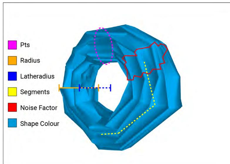
Figure 8: Torus shape and parameters
